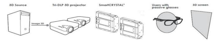
Most types of 3D cinema projectors are compatible with the SmartCrystal™ Diamond Dual system.
