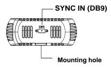
Power on emitter by using power supply adapter : LED will be off Connect synchronization cable to emitter: If a signal coming from projector is detected (2D or 3D mode), LED will be fixed red
