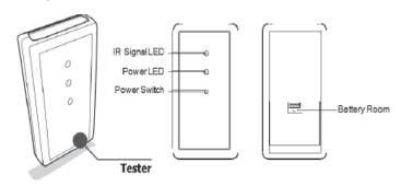
Active 3D Glasses VAIK-0300 is a handy unit to be carried by a cinema technician to check performance of 3D glasses. Turn on the power, then the tester emits low rate IR signal to activate 3D glasses. Working 3D glasses will then show a flickering.
