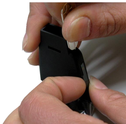
BATTERY TOOL to unlock the battery
