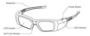
Charge the 3D glasses: Please charge your 3D glasses by connecting the 3D glasses to the USB port of your computer or the 3D glasses charger (sold separately) with supplied USB charging cable when they give low battery warning. Red LED indicator will keep lighting on until the charging is finished. A full charge may take 4 hours.
