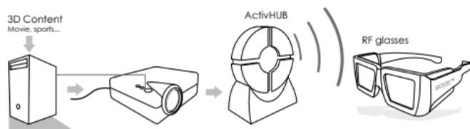
**The ActivHub™ RF50 can transmit RF synchronization when receiving an IR 3D signal.**
