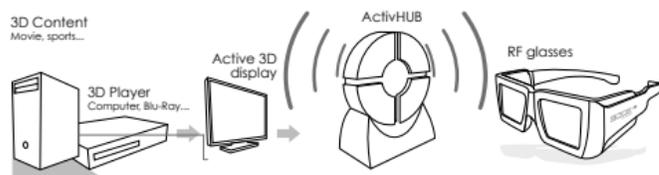
**The ActivHub™ RF50 can transmit RF synchronization when receiving a DLP-Link™ 3D signal.**
